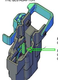
REINSERT SLIDE PAD IN SAME ORIENTATION AS REMOVED
