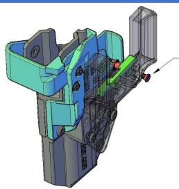
UNSCREW FASTENERS AND REMOVE BELT BAR FROM THE DROP MOUNT SLOT
