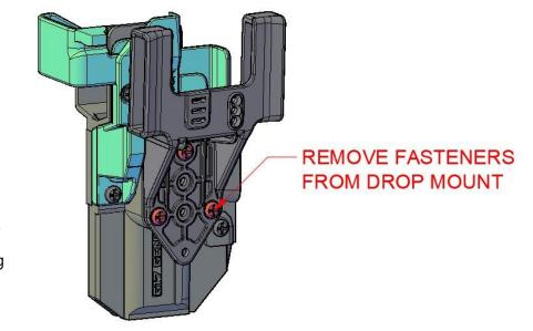
Flat screwdriver or an offset screwdriver may be of assistance during this procedure.
