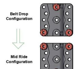
Adjust hardware on **Slide Pad** to match as displayed.
