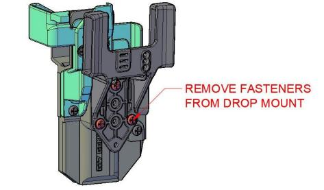
Flat screwdriver or an offset screwdriver may be of assistance during this procedure.
