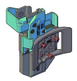
FASTEN MID RIDE ONTO HOLSTER USING THE SAME SCREWS THAT WERE ATTACHED TO THE DROP MOUNT
