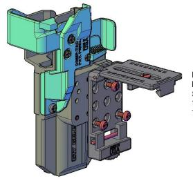
FASTEN PLM ONTO HOLSTER USING THE SAME SCREWS THAT WERE ATTACHED TO THE DROP MOUNT
