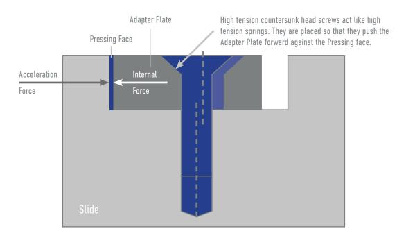
The highest stress/load for the slide and all mounted parts results from the acceleration of the slide while firing a round. The acceleration can go up to 1800 G. The force on the Adapter Plate which results from this effect is transferred over the Pressing Face from the Adapter Plate to the Slide. The design of the whole system is so that the Adapter plate is always pressed against this transfer Surface.
